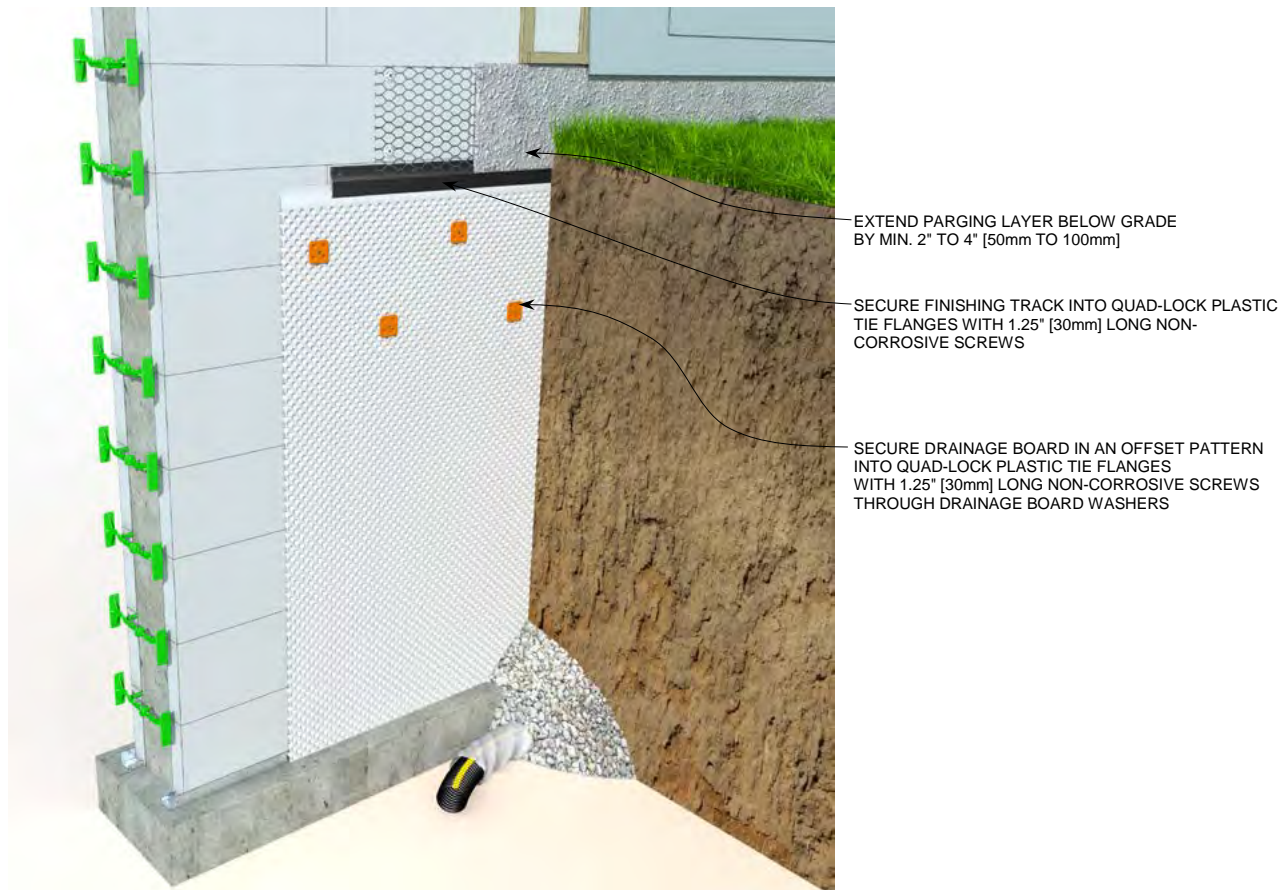
Figure 134: Damp Proofing with Drainage/Dimple Board
