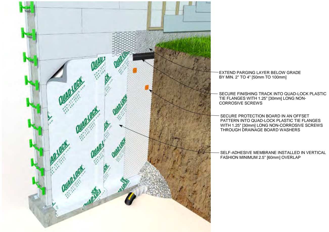
Figure 135: Water Proofing with Protection Board
