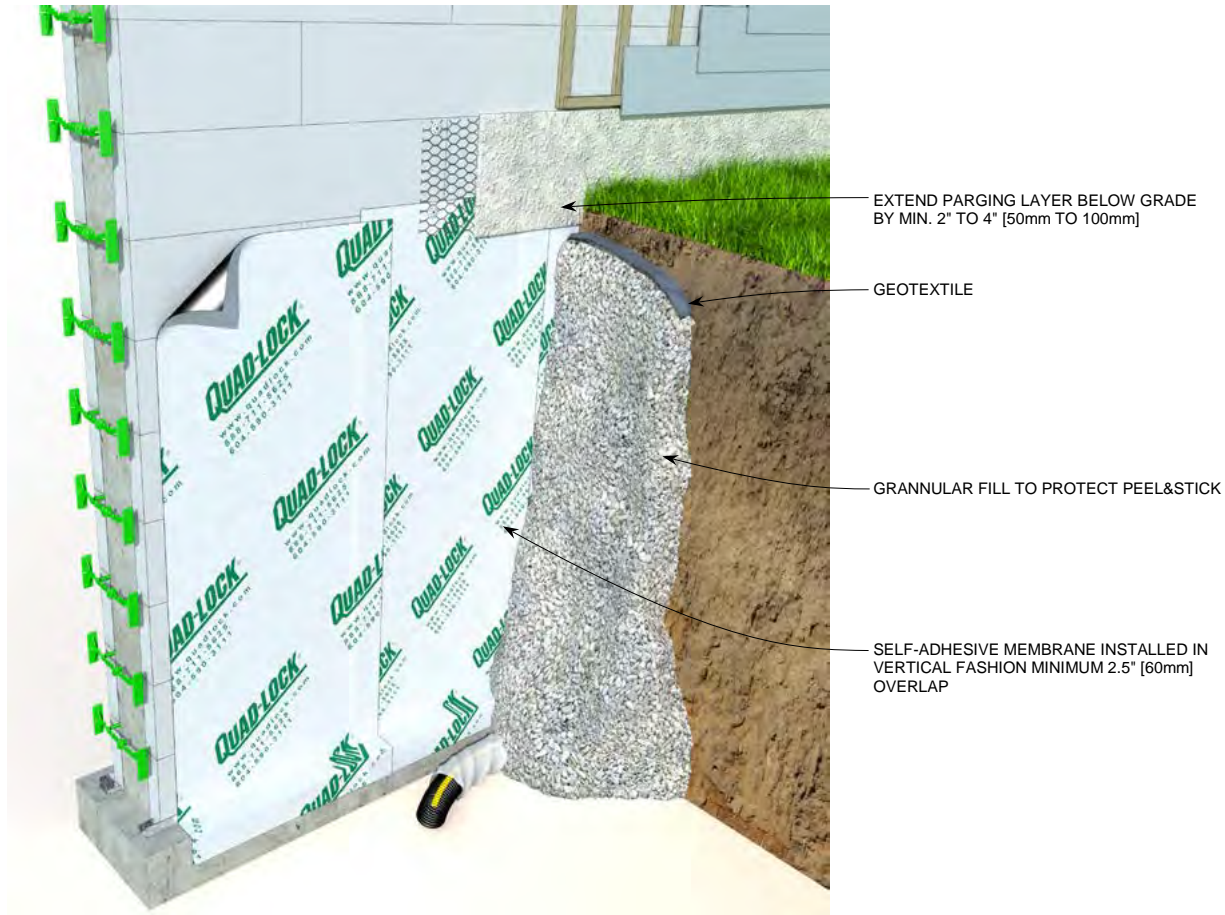
Figure 136: Water Proofing with Peel&Stick
